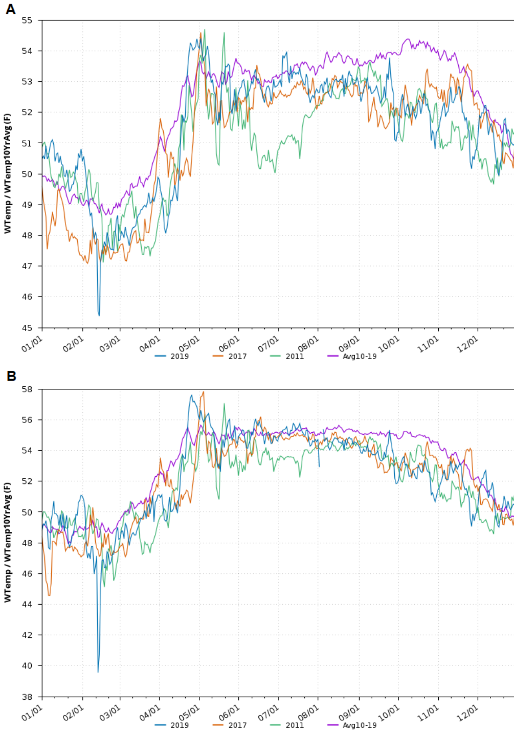
Water temperatures in 2019 at the Clear Creek confluence gage (upper panel; CCR, RM 292) and the TCP at Balls Ferry Bridge gage (lower panel; BSF, RM 275). Temperatures for 2017, 2011, and the 10-year average are also shown. There is no temperature monitor at the pilot TCP of Airport Road Bridge (RM 284) located between the two compliance locations. Figure and data from SacPAS (2020).
